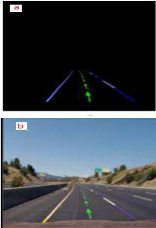
Fig.7 (a) Result after returning to the camera view. (b) Superposition of the result on the original image algorithm/
