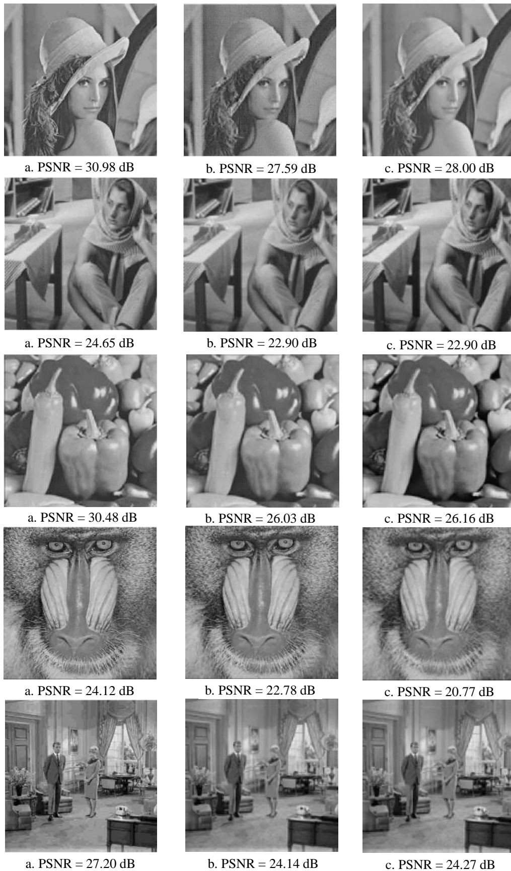
Fig. 4. Reconstructed Lena, Barbara, Peppers, Baboon and Living room test images given at bitrate of 0.26 bpp. (a) Exact DCT [17]. (b) Zonal BinDCT-C8 [15]. (c) Proposed method.
