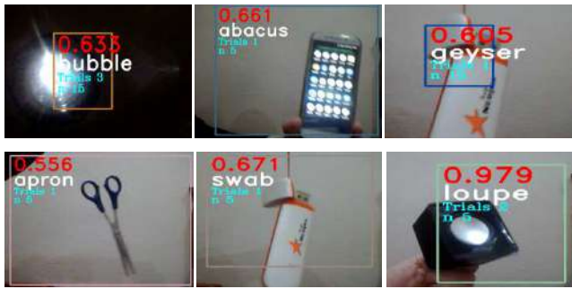
Fig. 14. Erroneous detections with static camera.
