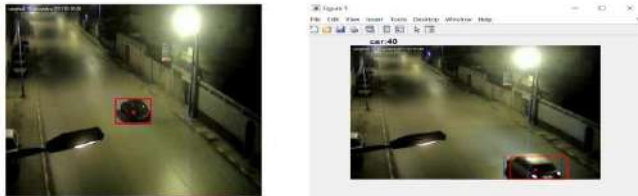
Fig. 7. Results of Kalman filter tracking.
